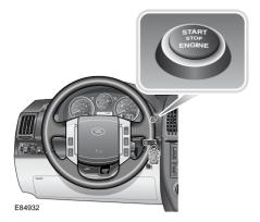
The start/stop button is used to start or stop the engine, or to turn on the ignition without starting the engine.
