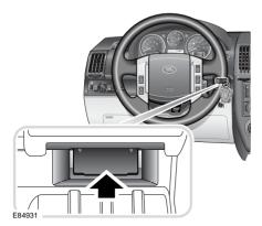
Before the engine can be started, the remote control will need to be docked with the buttons facing upwards.
